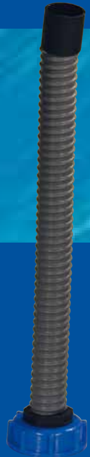
Wastewater cap DIN 51 incl. 30 cm wastewater hose with connection piece inner-Ø 28 mm Article code 8291.01.00
