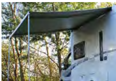
A 12V motor pushes Freedom's folding arms out to extend the lead rail.
